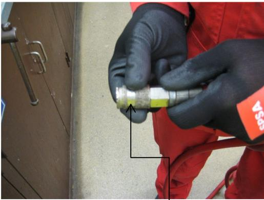
The shroud should now be checked and should be free to rotate
