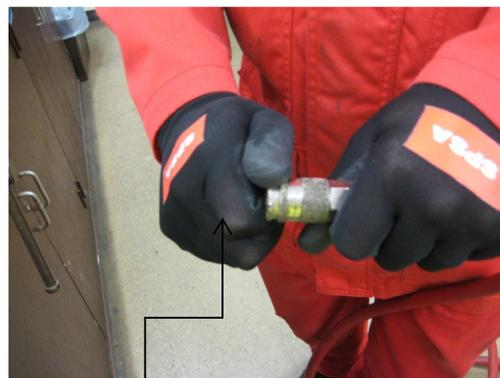
Try and twist the end. No movement should be observed.
