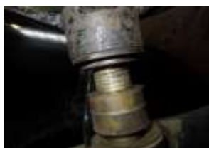
Worn threaded bolt
