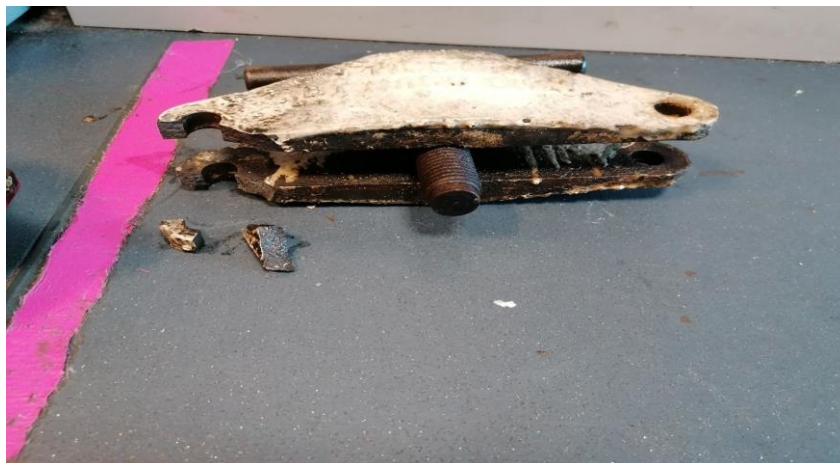
Filter broken casting
