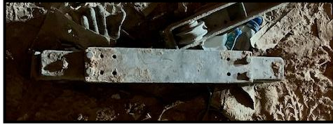
Runner – positioned between footplate and track. Securing clamps not available.
